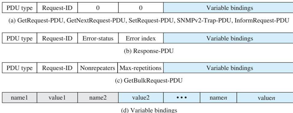
**Figure 20.6** SNMPv2 PDU Format
