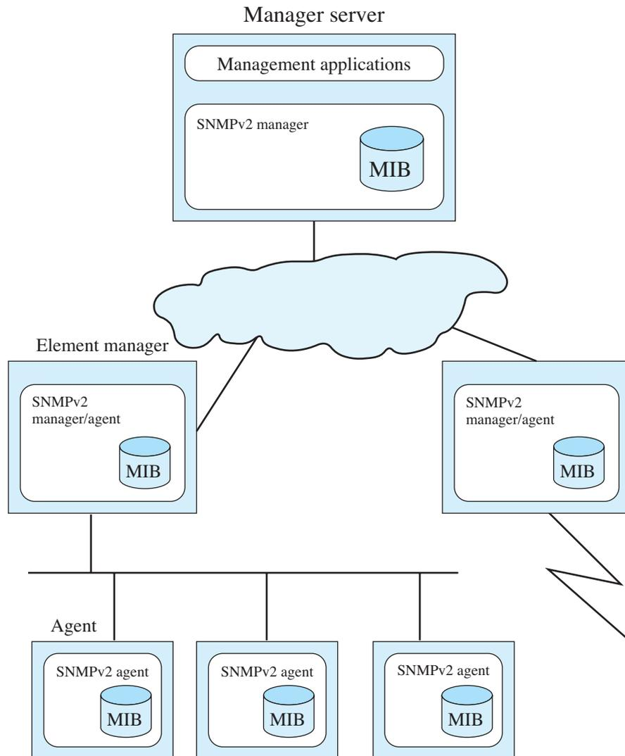
**Figure 20.5** SNMPv2-Managed Configuration
