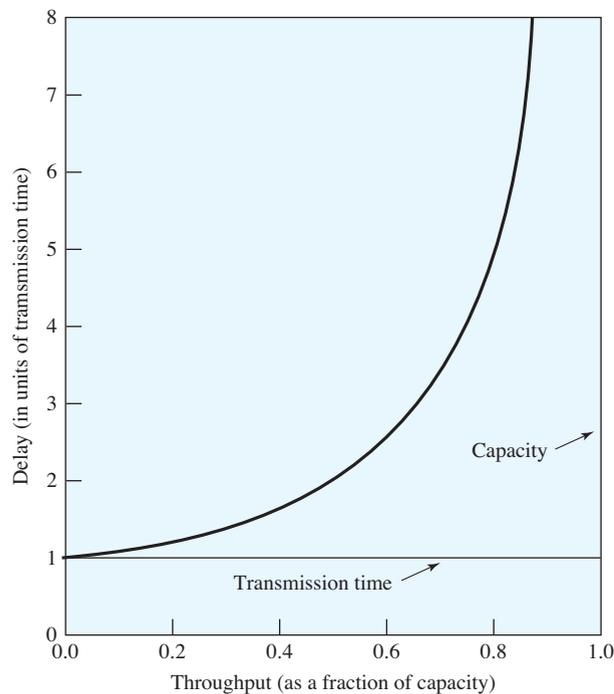
**Figure 21.5** Throughput Delay
